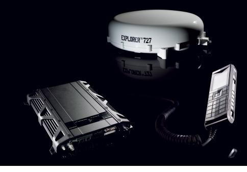
Composed of three units (a transceiver, a IP handset and an antenna), the Explorer 727 is the high-end BGAN solution for vehicles as it provides on the move high-speed Internet and phone networks access. It offers voice and data interfaces including ISDN and 4 Ethernet ports, ideal for multiple users while travelling in their vehicles.
